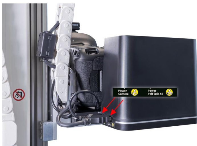
Fig. 9: Cable connections of PolFlash XE DX2 and camera to ATBM Tower (viewed from the right)
