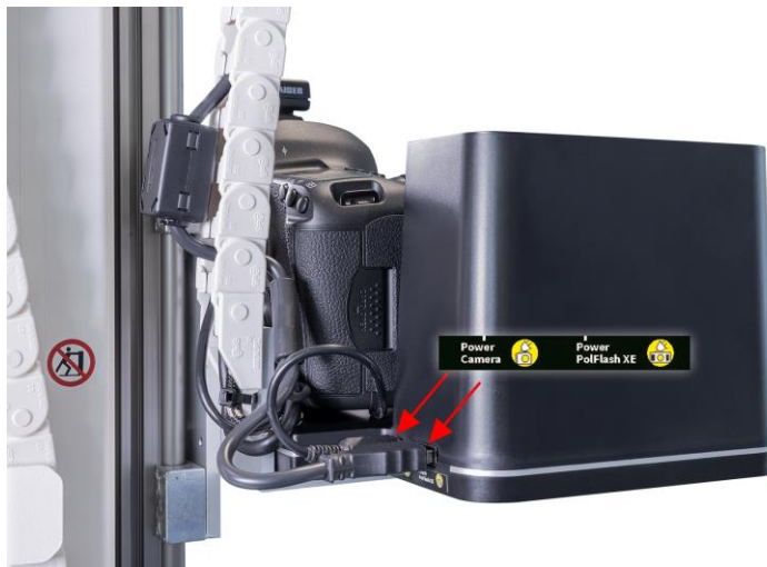
Fig. 10: Cable connections of PoIFlash XE DX2 and camera to ATBM Tower (viewed from the right)
