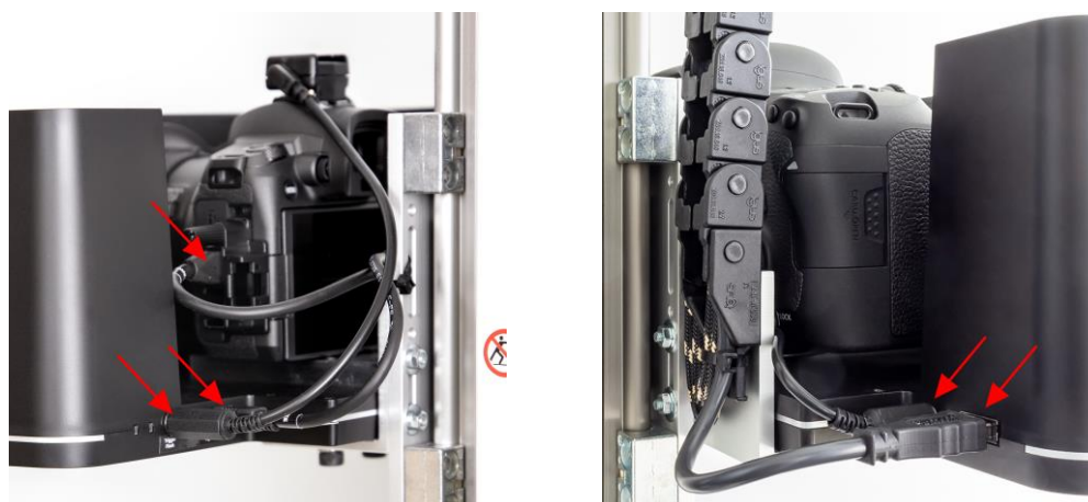
Fig. 13: Cable connections of PoIFlash XE and camera to ATBM Tower (viewed from the left and right)
