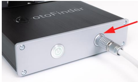
Fig. 14: Push-Pull round plug connection with the medicam cable on the Docking Station
