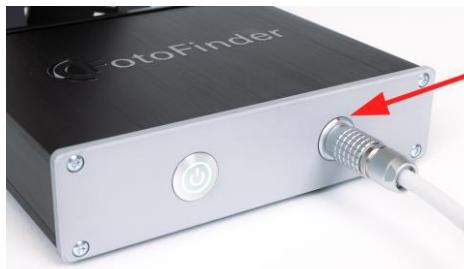
*Fig. 14: Conexāo de plugue redondo push-pull com medicam na Docking Station*
